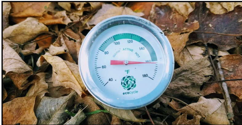
A long-stemmed thermometer can take the temperature at the center of a compost pile.
